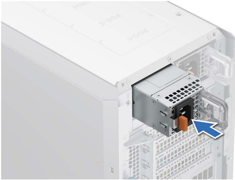
Figure 79. Installing a power supply unit
