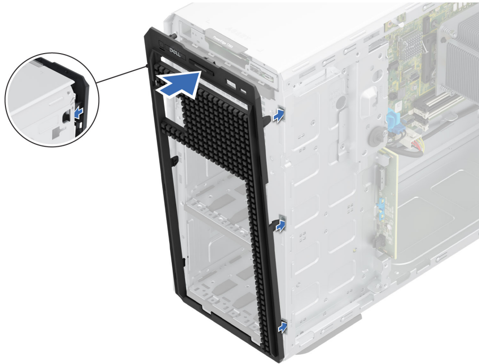
Figure 97. Installing the front faceplate
