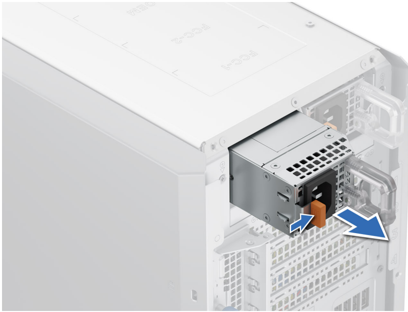
Figure 78. Removing a power supply unit
