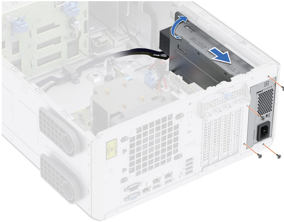
Figure 83. Installing the PSU cage
