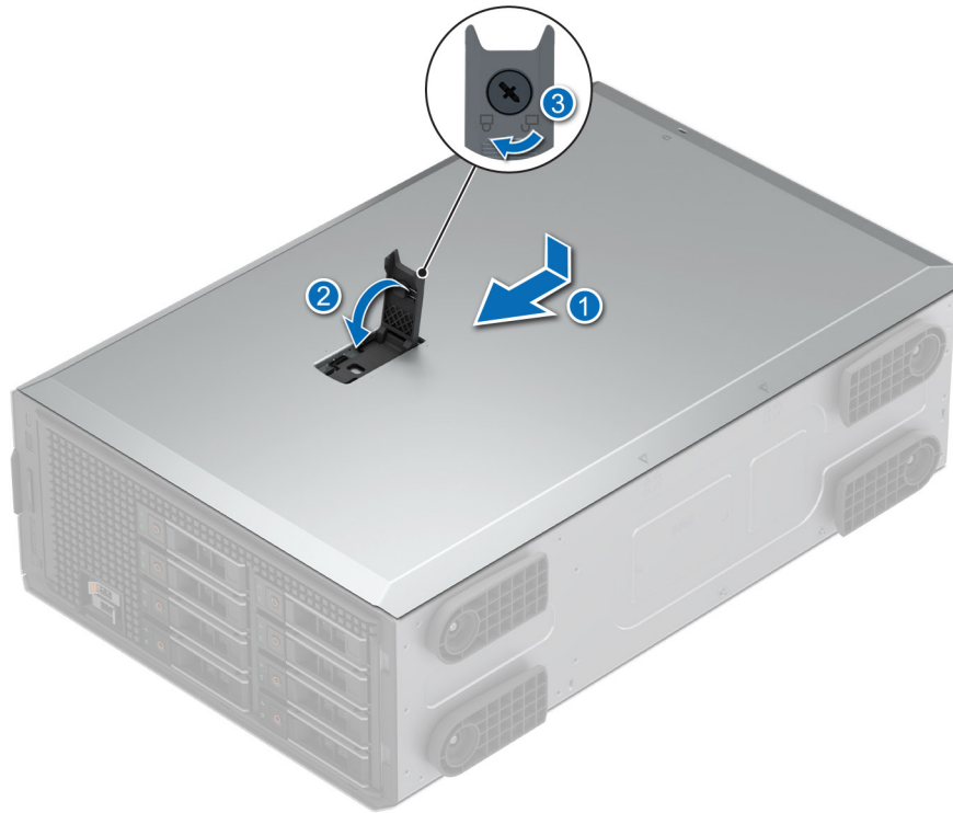
Figure 17. Installing the system cover
