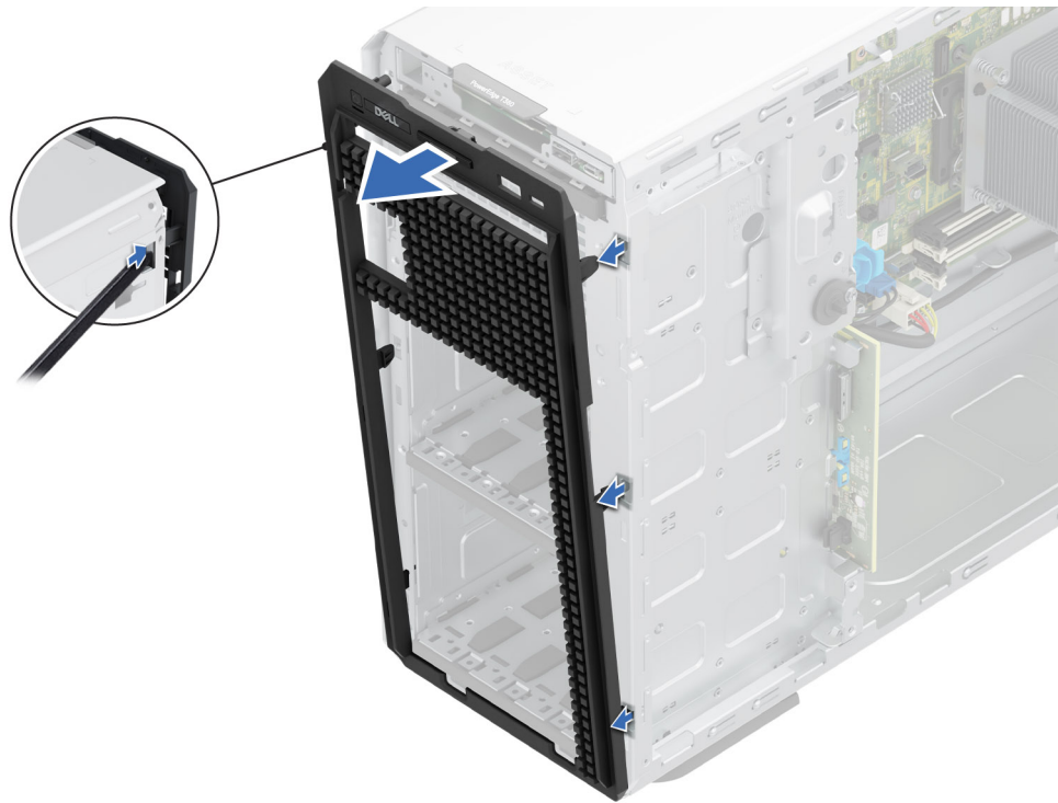
Figure 92. Removing the front faceplate
