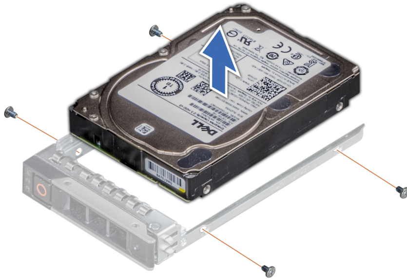
Figure 28. Removing the drive from the drive carrier
