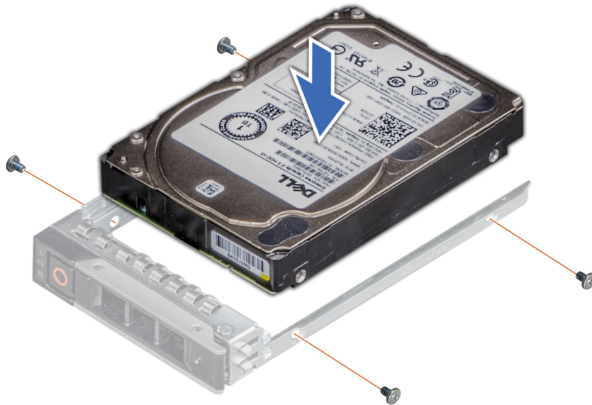
Figure 29. Installing a drive into the drive carrier
