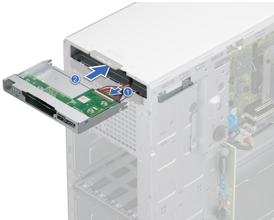
Figure 96. Installing the control panel cage
