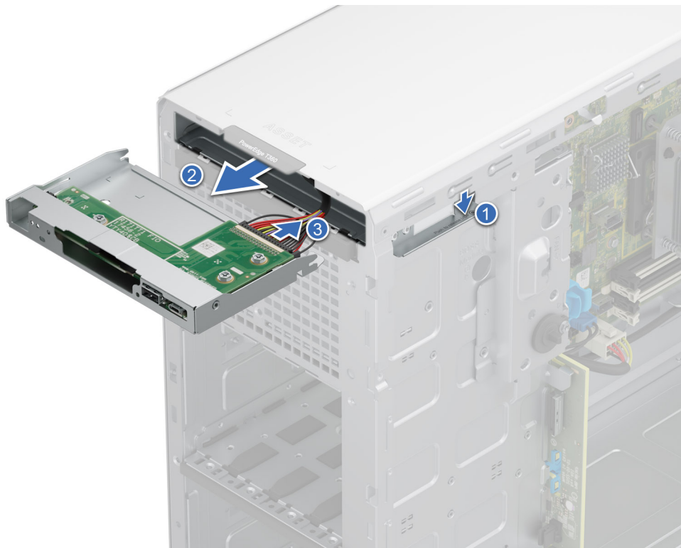
Figure 93. Removing the control panel cage
