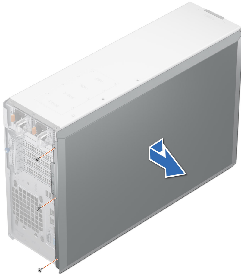
Figure 91. Removing the system side cover
