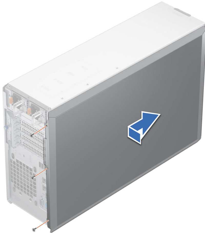
Figure 98. Installing the system side cover
