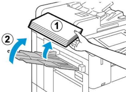
2. To open Door A, lift the release lever, then open Door A.
