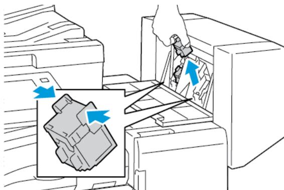
4. Hold the tabs on both sides of the new staple cartridge and insert the cartridge into the original position in the finisher.
