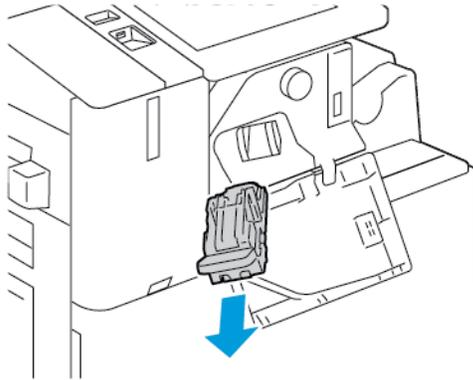
3. Check inside the finisher for any loose staples, then remove the staples.
