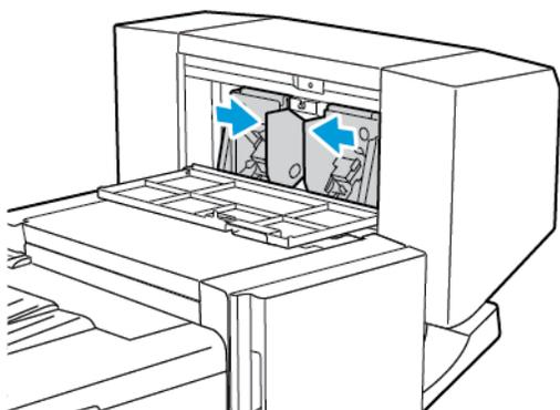
3. Hold the tabs on both sides of the staple cartridge and pull the cartridge out of the finisher.
