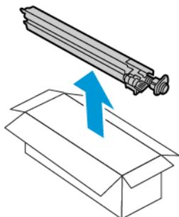
**!** **Caution:** Do not touch the surface of the transfer belt cleaner. This action can cause image quality to deteriorate.
