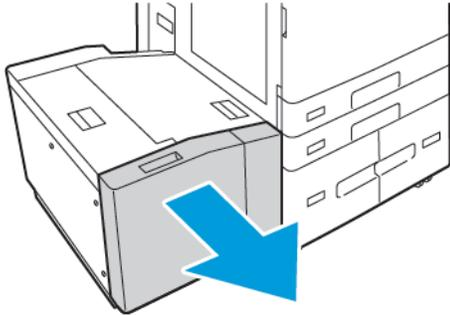
2. Open the side gate. Remove the screw that holds the spacer plate at the back of the tray, then lift the spacer plate out of the tray. Repeat the procedure for the spacer plate at the front of the tray.
