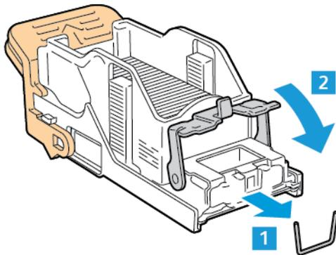
**⚠ WARNING:** The points of the jammed staples are sharp. Remove the jammed staples carefully.
