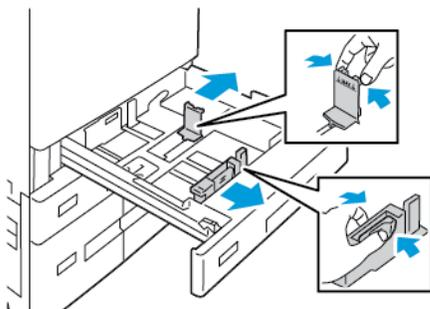
4. Flex the sheets back and forth and fan them, then align the edges of the stack on a level surface. The procedure separates any sheets that are stuck together and reduces the possibility of jams.
