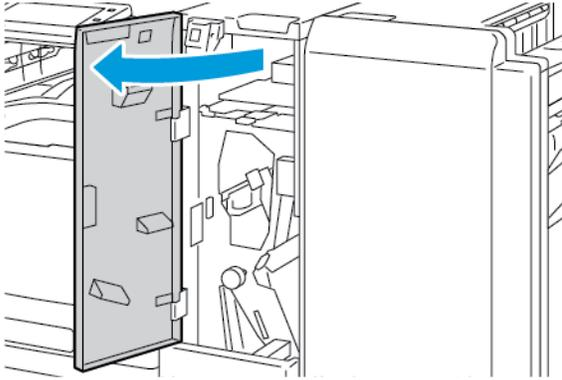
2. Open the folder tray, move lever 2e to the right, then carefully remove the paper.
