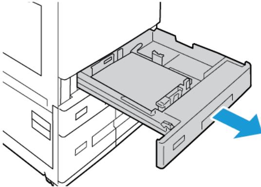
2. Remove any paper from the tray, pinch the guide levers, and move the guides outward until they stop.
