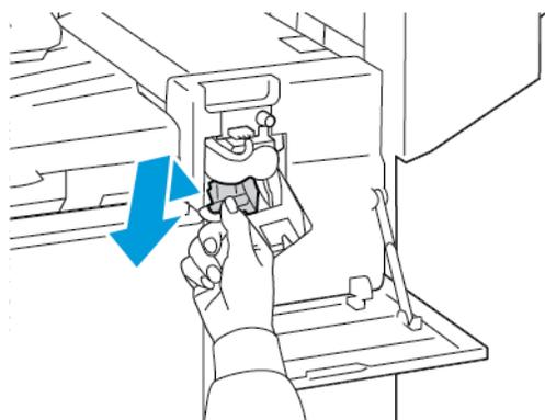
5. Check inside the finisher for any loose staples, then remove the staples.
