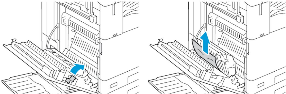
5. If paper is jammed in the fuser, remove the jammed paper from areas A1 and A2.
