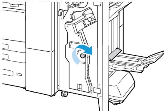
3. To remove the paper, pull the paper in the direction shown.
