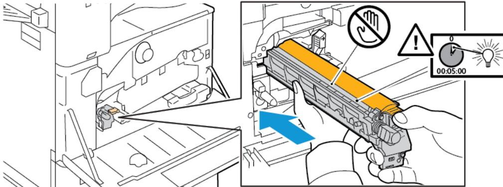
7. With the guides inserted in the slot, remove the black paper sheet. Remove the tape from the top of the cartridge shield.
