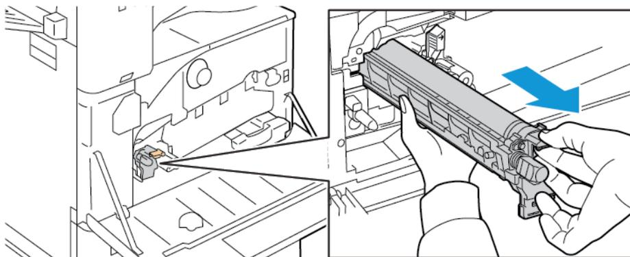
5. Remove the packing material from the end of the new drum cartridge.
