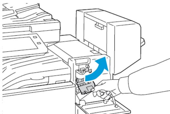
4. To remove the staple cartridge, grasp the orange handle, then pull it firmly toward you.
