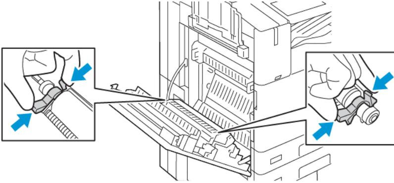
5. Lift the used transfer roller out of the printer.
