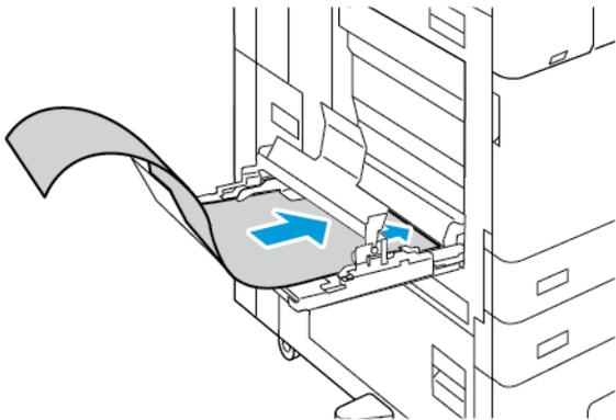
4. Carefully roll the remaining length of the banner paper into the Long Sheet Feed Extension guides. Ensure that the trailing edge rests against the front guide.
