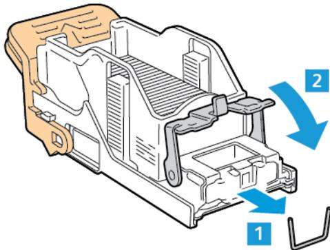
8. Grasp the orange handle, then insert the cartridge into the stapler assembly until the cartridge clicks into place.
