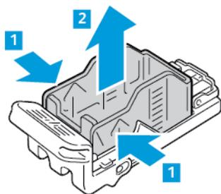
5. Insert the front side of the new staple pack into the staple cartridge, then push the rear side into the cartridge.
