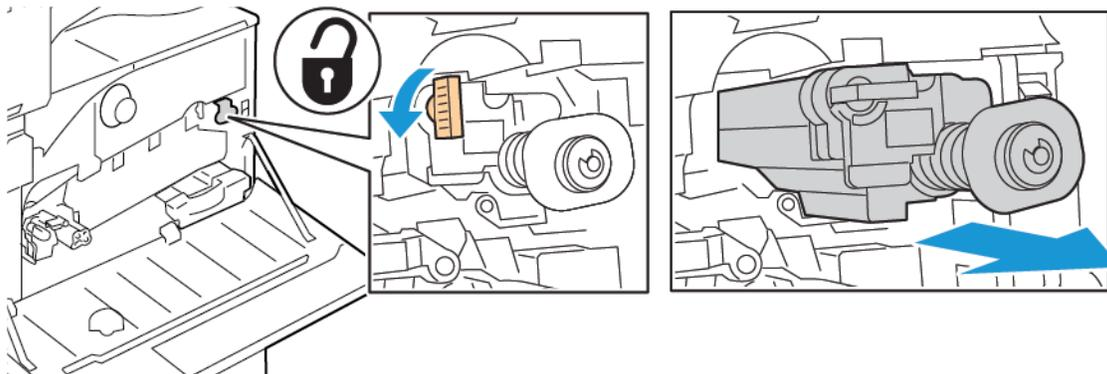
**!** **Caution:** Do not touch any toner adhering to the transfer belt cleaner. Do not tilt the transfer belt cleaner, toner can spill.
