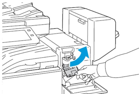
4. To remove the staple cartridge, grasp the orange handle, then pull the handle toward you.
