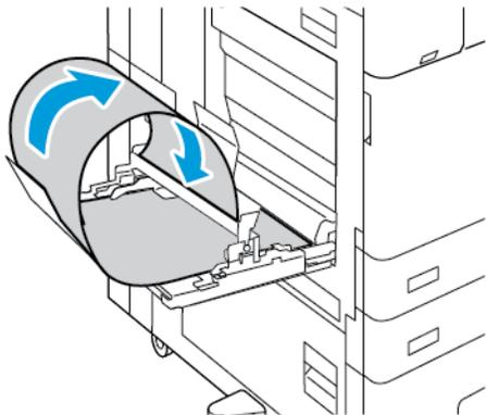
5. Adjust the Bypass Tray width guides until they touch the edges of the paper.
