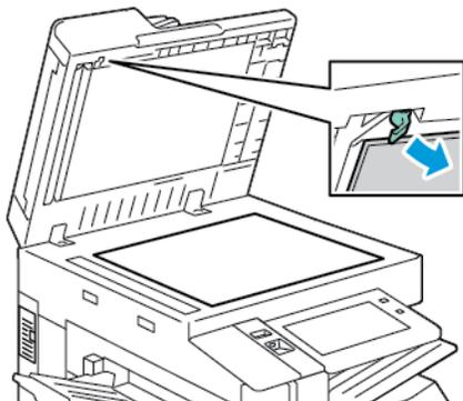
2. To separate the left end of the document cover from the lens assembly, continue to lower the lever.
