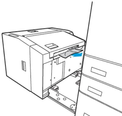
3. Open the top cover, lift the inner cover, then remove any jammed paper in the direction shown.
