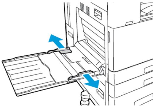
3. Load the banner paper in the tray. Load the paper with the short edge leading into the printer.
