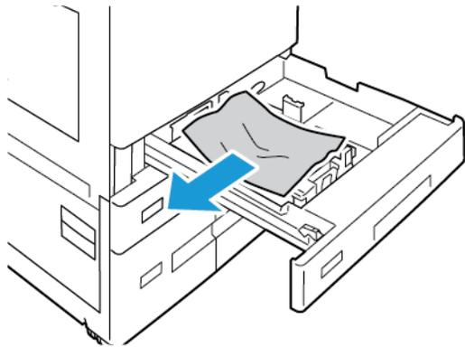
4. If the paper is torn, remove the tray completely, then check inside the printer for torn pieces of paper.
