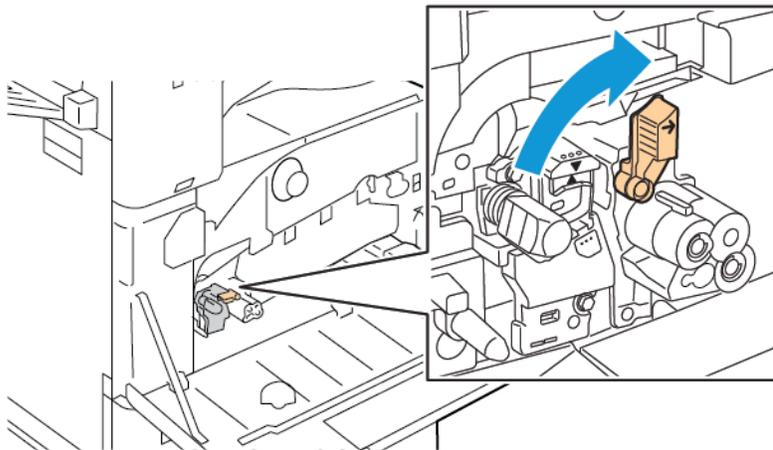
4. Grip the orange handle of the drum cartridge as shown, then pull the drum cartridge straight out of the printer. Place the used drum cartridge in the plastic bag, then place the bag in the box.
