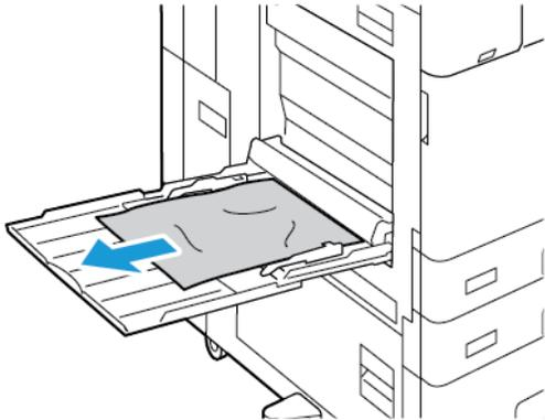
2. If the paper is torn, check inside the printer for torn pieces of paper.
