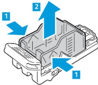
6. Insert the front side of the new staple pack into the staple cartridge, then push the rear side into the cartridge.
