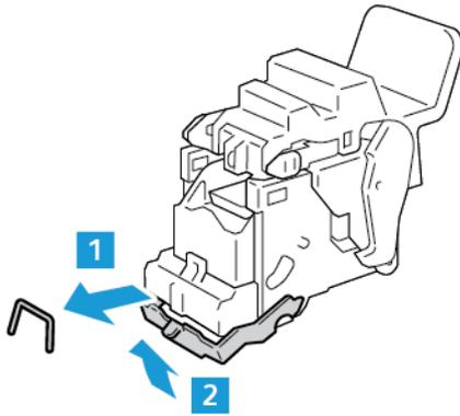
9. To return the staple cartridge to the booklet maker, insert the staple cartridge, then push up on the cartridge handle as shown.
