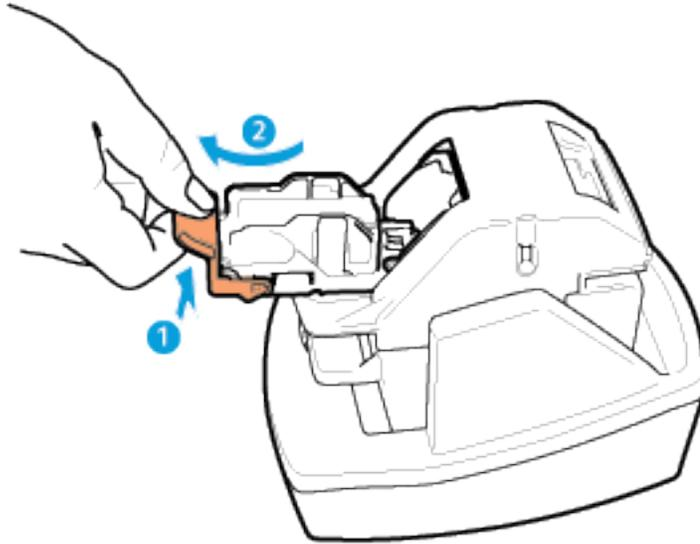
3. Unpack the new staple cartridge. Remove any partial strips and any staple strips that are not flat.
