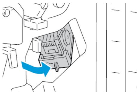
3. To remove the staple cartridge, grasp the orange handle, then pull it firmly toward you.
