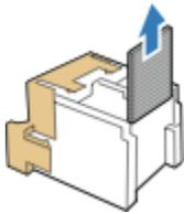
5. Hold the tabs on both sides of the staple cartridge and insert the cartridge into the original position in the finisher.
