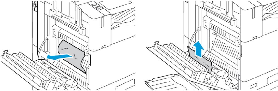
4. If paper is jammed on the inside of door A, lift handle A3, then remove the jammed paper. Return handle A3 to the original position.
