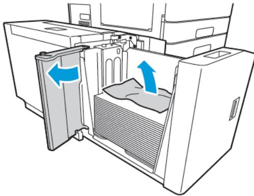
7. Reload the tray with undamaged paper, close the side gate, then close the tray.
