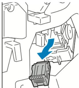
4. Pinch both sides of the staple pack and remove the staple pack from the cartridge.
