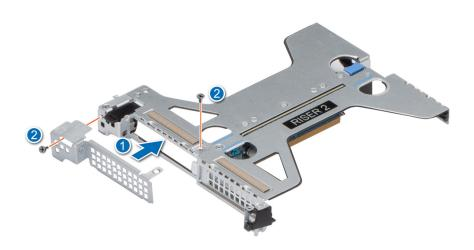
Figure 73. Installing the PCIe blank
