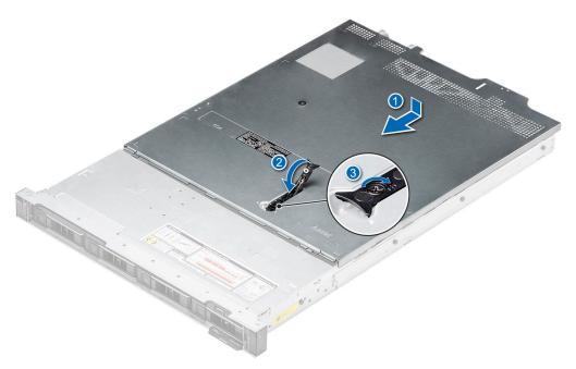
Figure 18. Installing the system cover
