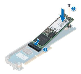
Figure 81. Installing the M.2 SSD module
