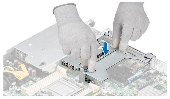
Figure 63. Installing the Riser 2c
