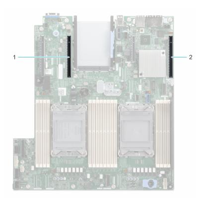
Figure 57. Expansion card slot connectors
