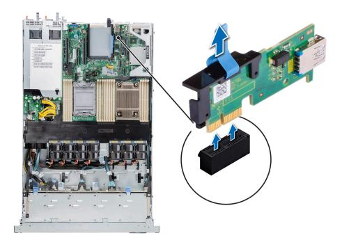
Figure 90. Removing the internal USB card
