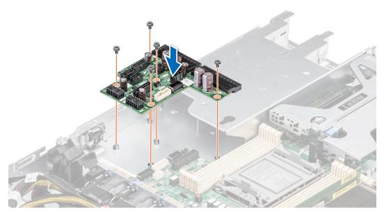
Figure 99. Installing the power interposer board
