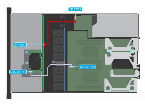
Figure 40. Cable routing -  $4 \times 3.5$ -inch drive SAS or SATA backplane with ODD, Butterfly riser, BOSS and SNAPI riser
