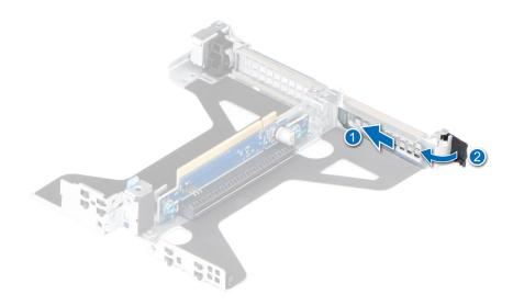
Figure 67. Installing filler bracket in the Riser 2c
