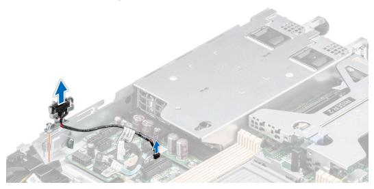
Figure 25. Removing the intrusion switch module
