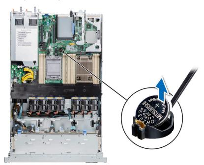
Figure 88. Removing the system battery
