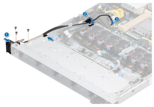
Figure 104. Installing the left control panel
