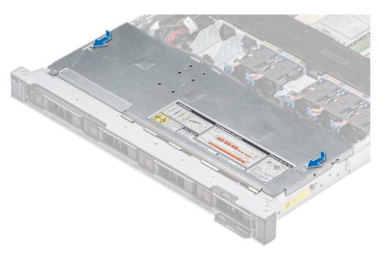
Figure 20. Installing the drive backplane cover
