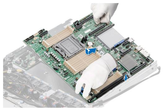
Figure 101. Installing the system board
