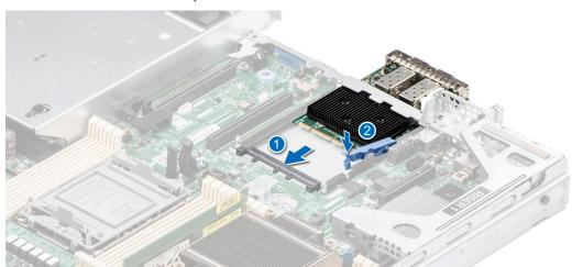
Figure 83. Installing the OCP card
