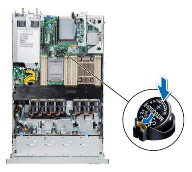
Figure 89. Installing the system battery
