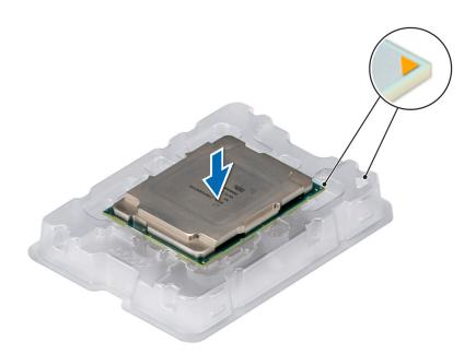
Figure 48. Aligning pin 1 marks of processor with tray
