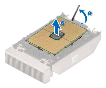
Figure 47. Lift the TIM break lever
