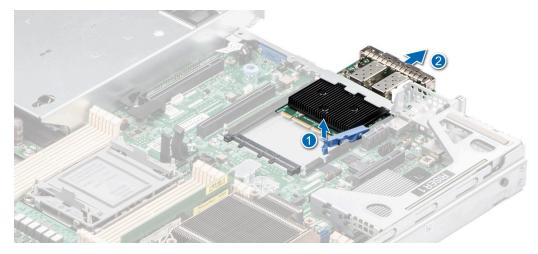
Figure 82. Removing the OCP card
