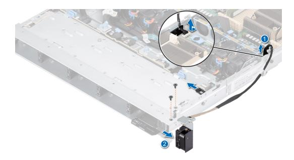
Figure 105. Removing the right control panel
