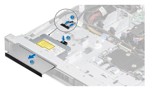
Figure 33. Removing the optical drive
