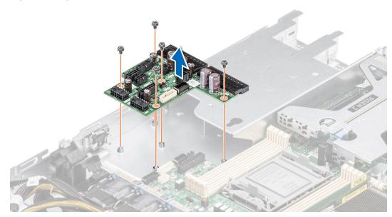
Figure 98. Removing the power interposer board
