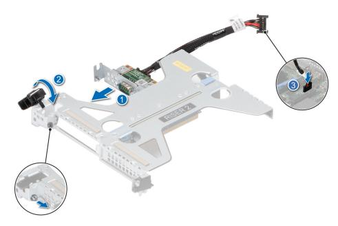
Figure 75. Installing the Serial COM port
