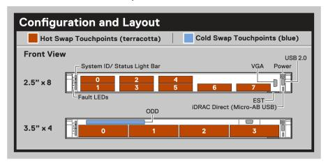
Figure 6. R450 Configuration and layout
