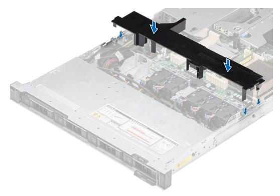
Figure 22. Installing the air shroud
