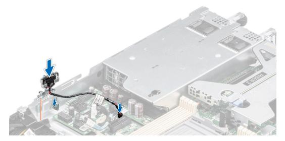
Figure 26. Installing the intrusion switch
