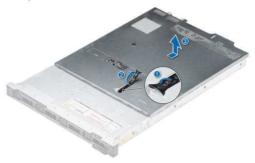
Figure 17. Removing the system cover
