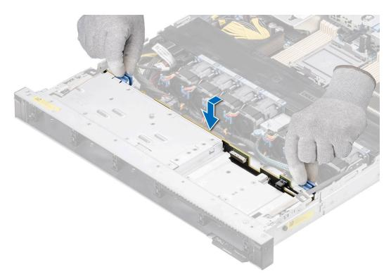
Figure 38. Installing the drive backplane
