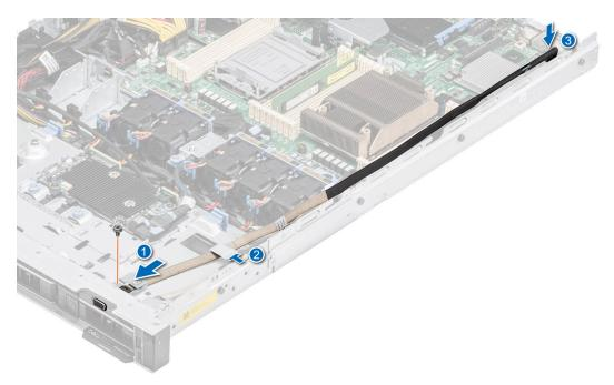
Figure 93. Installing the VGA module
