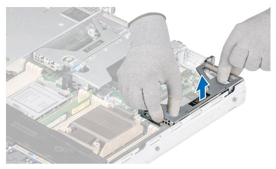
Figure 60. Removing the Riser 1
