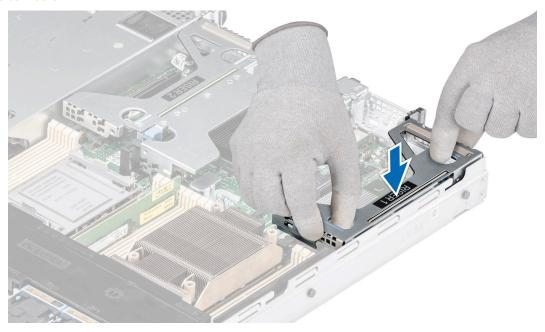
Figure 62. Installing the Riser 1
