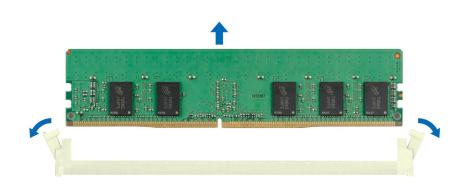
Figure 43. Removing a memory module
