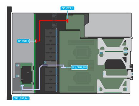
Figure 39. Cable routing - 8 x 2.5-inch drive SAS or SATA backplane with Butterfly riser, BOSS and SNAPI riser
