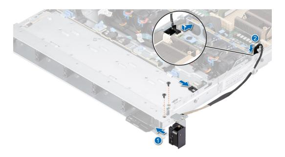
Figure 106. Installing the right control panel
