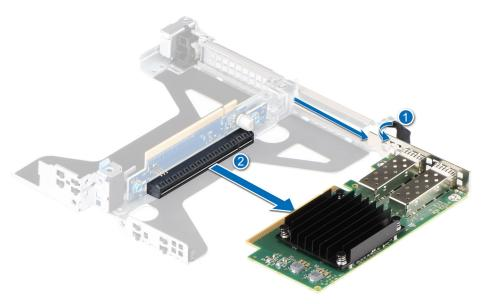
Figure 65. Removing an expansion card from Riser 2c
