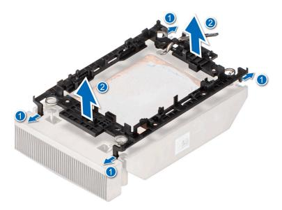
Figure 49. Removing the processor carrier
