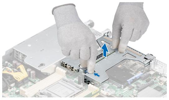
Figure 61. Removing the Riser 2c
