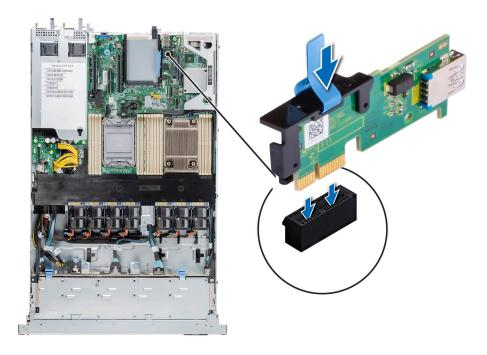
Figure 91. Installing the internal USB card
