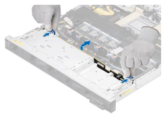
Figure 37. Removing the backplane
