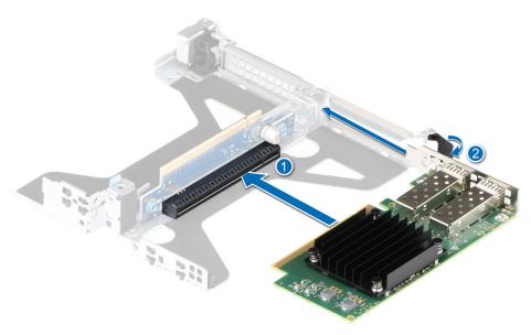
Figure 71. Installing an expansion card into a Riser 2c
