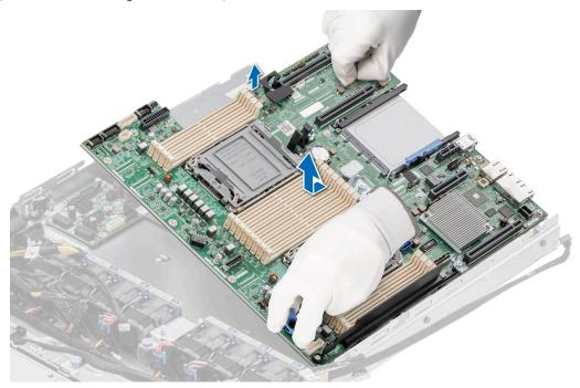
Figure 100. Removing the system board
