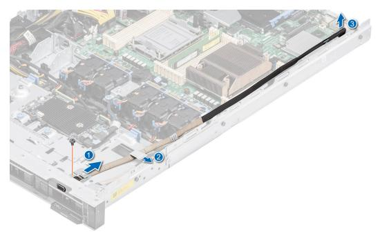
Figure 92. Removing the VGA module
