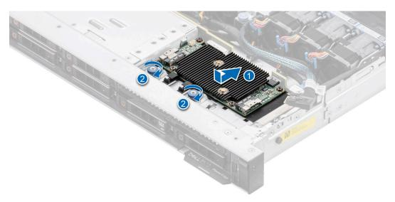
Figure 87. Installing the front mounting front PERC module for 8x2.5-inch system
