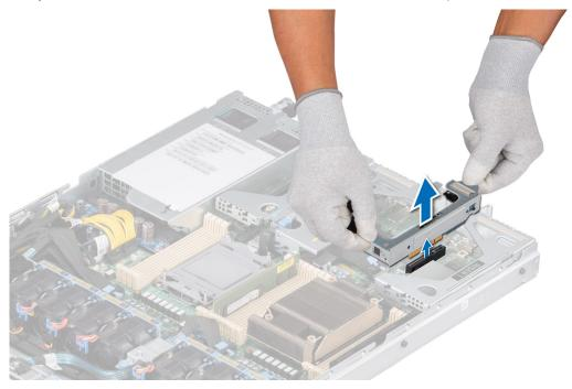
Figure 76. Removing the M.2 BOSS riser
