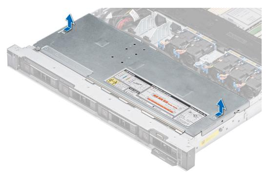
Figure 19. Removing the drive backplane cover
