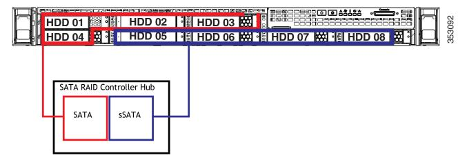
■ Each controller is listed separately in the BIOS. You can select the boot order of the controllers in the BIOS (use the Boot Options tab in the BIOS Setup Utility).
