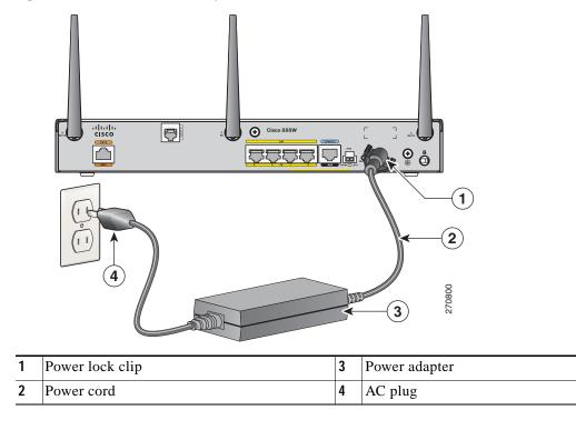
Figure 3-35 Power Lock Clip Latched Into the Holes on Either Side of the Power Connector
