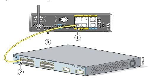
Figure 3-2 Connecting to an Ethernet Switch
