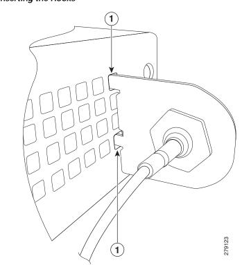
Figure 3-22 Inserting the Hooks
