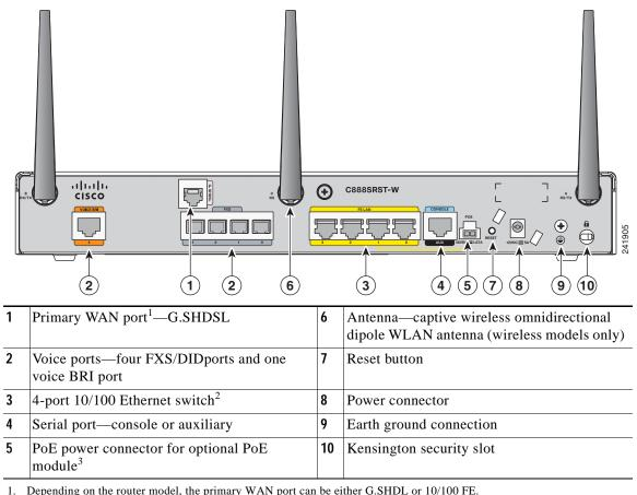
Figure 1-24 Back Panel of the Cisco C888SRST-W Voice Router
