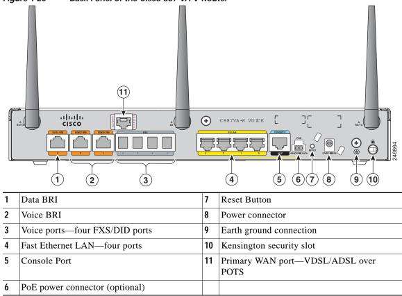
Figure 1-26 Back Panel of the Cisco 887 VA-V Router
