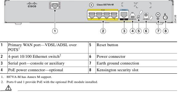
For the Cisco 887VA, the primary WAN port is designed for an RJ-11 connector only. Damage to the primary WAN port may occur if a non-RJ-11 connector is inserted.
