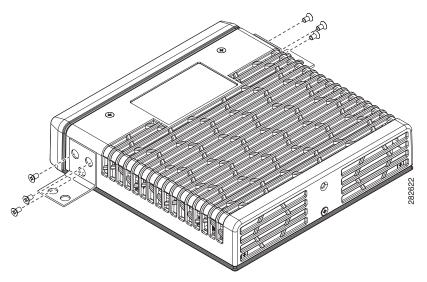
Step 3 Install the router to a wall stud using two number-10 wood screws, round- or pan-head, with number-10 washers or two number-10 washer-head screws. The screws must be long enough to penetrate at least 1.0 inch (25.4 mm) into the supporting wood or metal wall stud. (See Figure 2-22.)
