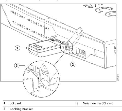
Figure 3-15 Installing the Locking Bracket
