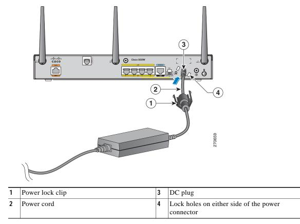
Figure 3-34 Securing the Power Cord
