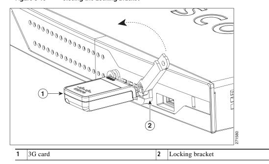
Figure 3-16 Closing the Locking Bracket
