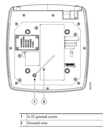
Figure 2-17 Connecting the Ring Lug onto the Grounding Point
