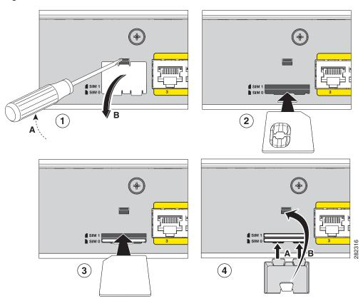
Figure 45 SIM Card Installation
