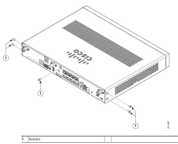
Step 2 Using the screws provided, attach the rack-mount brackets to the Cisco 890 series ISR chassis, as shown in Figure 2-44. Use two screws on each side. Use a number 2 Phillips screwdriver to install the bracket screws on both sides of the chassis.
