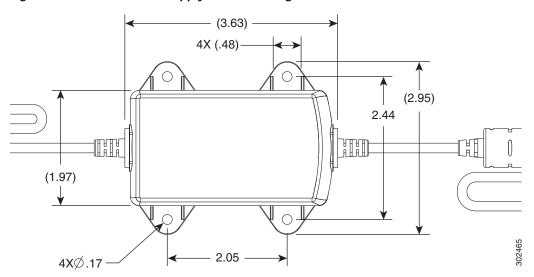
Figure 2-36 DC Power Supply Wall-Mounting Features
