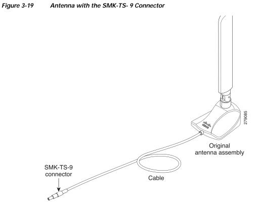
If you are using an extension cable, you must attach the 3G adapter for extended cable antenna to the body of the router. Depending on the SKU ordered, the adapters come with different connectors. Table 3-2 lists the different adapters and SKUs supported by each adapter. For instructions on how to install the adapter, see the "Installing the 3G Adapter for Extended Cable/Antenna" section on page 3-24. Otherwise, follow Step 7.
