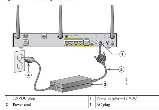
Figure 3-31 Connecting the AC Adapter
