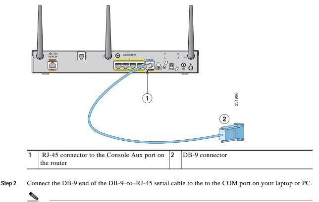
**Note** Some laptops and PCs do not come with DB-9 serial port connectors and may require a USB-to-serial port adapter.
