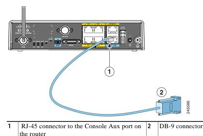
Step 2 Connect the DB-9 end of the DB-9-to-RJ-45 serial cable to the COM port on your laptop or PC.
