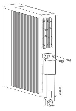
Step 2 Find the tab on the end of the DIN rail that extends past the router. (See Figure 2-24.) Press the tab in and slide the DIN rail out while the tab is pressed down.
