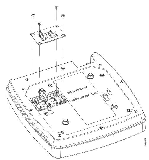
Figure 2-6 Accessing the SIM Card
