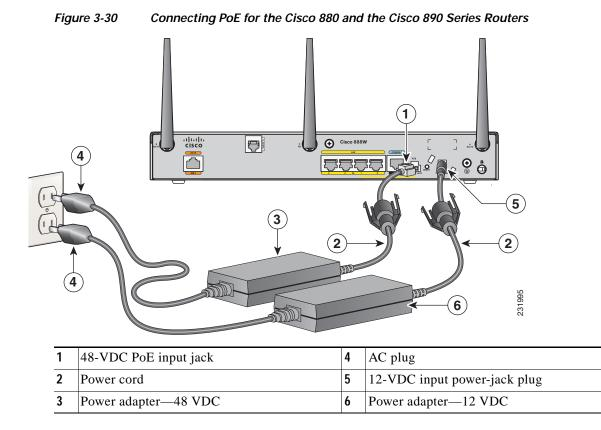
The Cisco 880 series ISRs with embedded WLAN antennas require a single external power supply: a 30-W power supply for non-POE-enabled routers or a 60-W power supply for POE-enabled routers. For the back panels of some of these routers, see Figure 1-29 and Figure 1-31.
