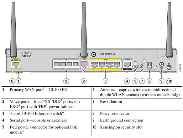
Figure 1-23 Back Panel of the Cisco C881SRST-W Voice Router
