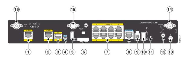
Figure 1-55 Back Panel of the Cisco C899G-LTE ISR
