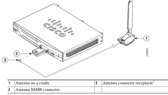
1. The antenna connector receptacle is located on either the left, right or front of the card for different SKUs. Please locate the receptacle of your card before plugging in the cable.
