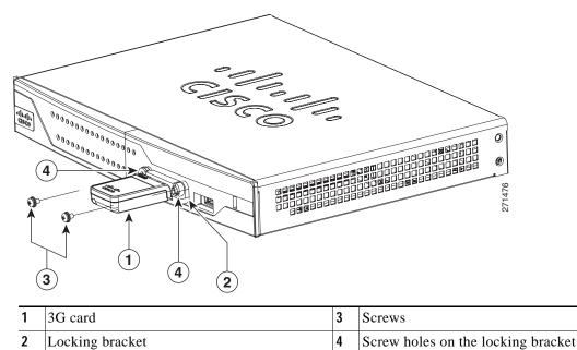
Figure 3-17 Inserting the Screws
