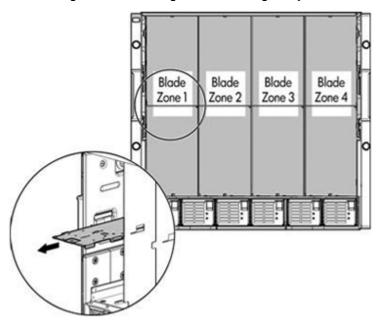
The BladeSystem c7000 enclosure is divided into 4 zones by the vertical support metalwork. Within each zone a removable divider is used to support half height devices. To install a full-height blade in any zone this divider must be removed. As a consequence a zone can only contain either full-height server blades or half-height server blades.
