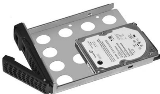
Disk tray with 2.5-inch HDD
