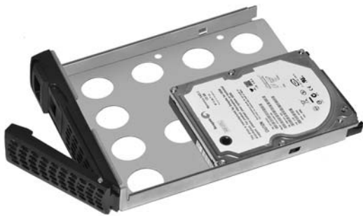
Disk tray with 2.5-inch HDD
