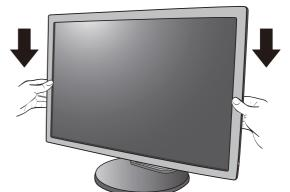
• Avoid placing hands on the upper or lower part of the height-adjustable stand or at the bottom of the monitor, as ascending or descending monitor might cause personal injuries. Keep children out of reach of the monitor while performing this operation.
