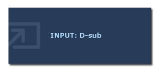
Press the **ENTER** key to toggle between different PC video signal inputs that may be connected to your monitor.
