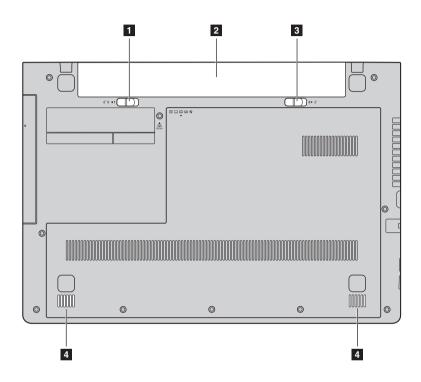
Battery pack latch - manual The manual battery pack latch is used to keep the battery pack secured in place.
