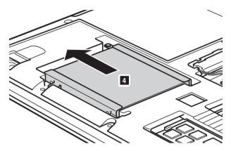
7 Take out the hard disk drive secured in a metal frame 5. Lenovo G40-30/G40-45/G40-70/G40-70m/Z40-70
