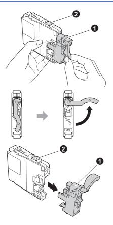
Install each ink cartridge in the direction of the arrow on the label.
