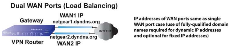
Figure B-8 Load Balancing for Dual Gateway WAN Ports
