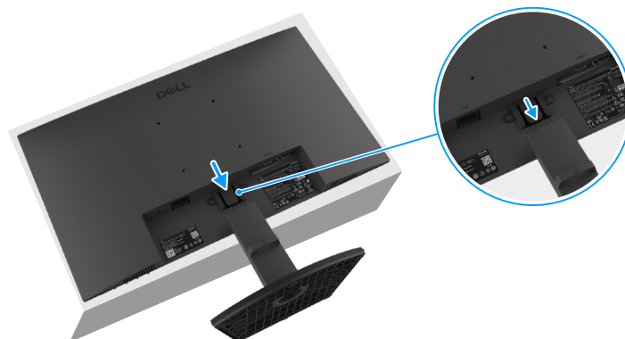
Figure 21. Remove the stand
