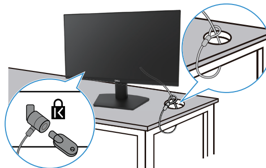
Figure 18. Using Kensington lock
