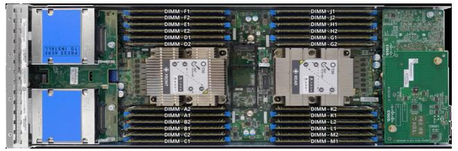
24 DIMMs, 6 Memory channels per CPU, up to 2 DIMMs per channel
