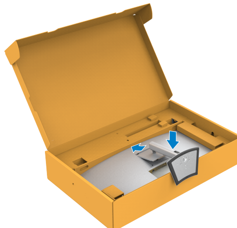
Figure 16. Insert the tabs on the stand riser into the slots
